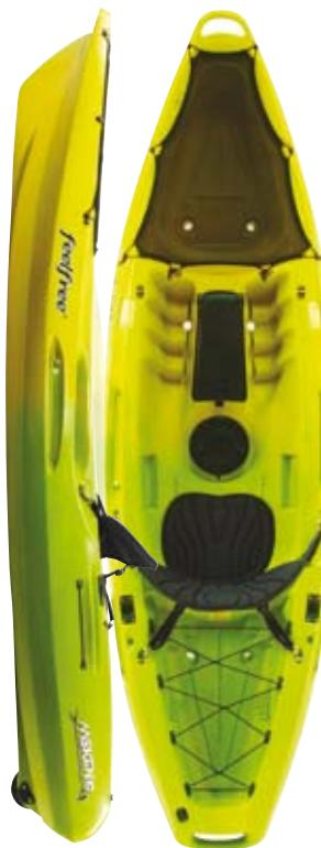
Length: 10: 315 cm / 10'3" - 12: 379 cm / 12'4" - width: 10: 89.5 cm / 35" - 12: 75 cm / 29" - weight: 10: 27.5 kg / 60.6 lbs - 12: 33 kg / 72.7 lbs - max. cap.: 10: 200 kg / 440 lbs - 12: 250 kg / 550 lbs
