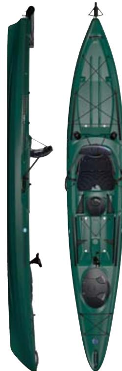
Length: 14' - 427 cm - Width: 28" - 71 cm - Max Capacity: 375 lbs - 170 kg - Weight: 75 lbs - 34 kg - Cockpit dims: 52" - 132 cm x 20" - 51 cm
