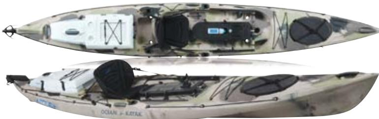
**Length: 4.7 m - width: 74 cm - weight: 35 kg - max. cap.: 250 kg**
