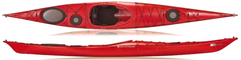
Length: 15'6" / 472 cm - width: 22.5" / 57 cm - weight: 52 lbs / 24 kg - max. cap.: 275 lbs / 125 kg
