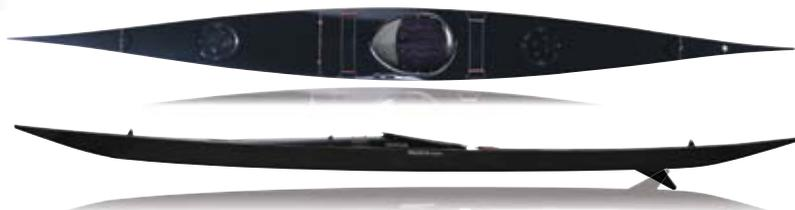
Length: 559 cm (18'4") - width: 52 cm (20'5") - volume: 259 L (68,4 US gal) - weight: 21 kg (46 lbs) - max. cap.: 136 kg
